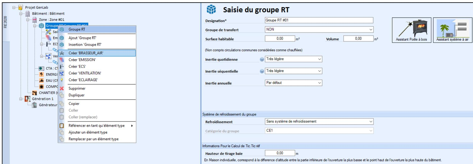
The screenshot displays the software interface for creating an air heater. On the left, a project tree shows the hierarchy: 'Projet GenLab' > 'Bâtiment : Bâtiment' > 'Zone : Zone #01' > 'Groupe RT'. A context menu is open over the 'Groupe RT' element, with 'Créer 'BRASSEUR\_AIR'' selected. The main window is titled 'Saisie du groupe RT' and contains the following fields:
